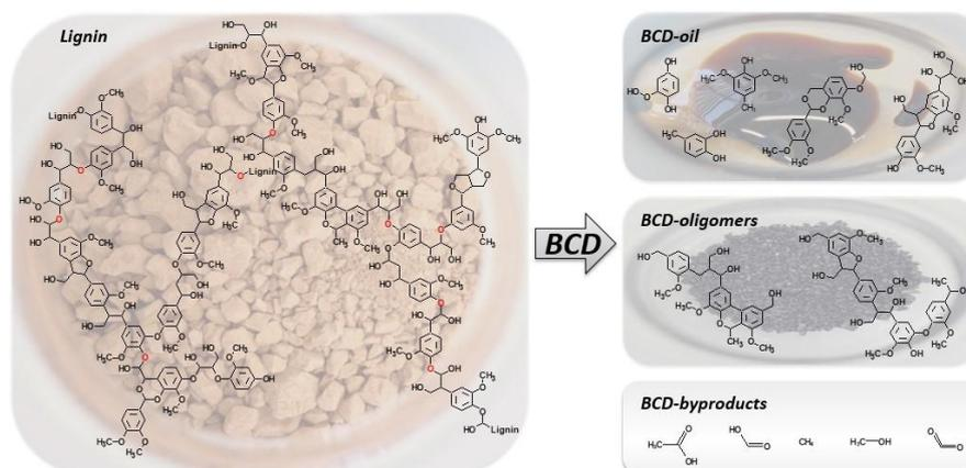
**Figure 2:** Reaction scheme for the base catalyzed depolymerization of Lignin [4].
