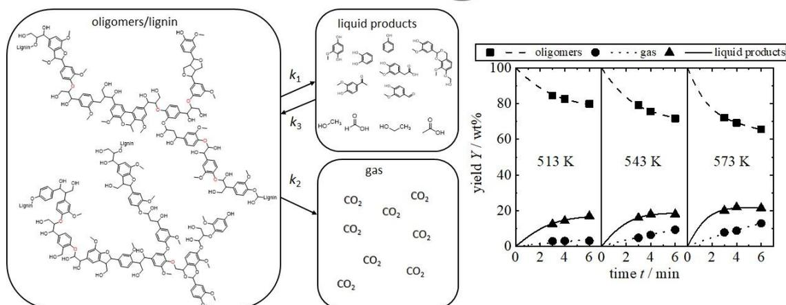
**Figure 4:** Proposed simplified reaction network (left) and comparison between the time-dependent model fit (lines) of oligomers, liquid products and gas and their experimental values (symbols), 1.67 wt.% NaOH, 5 wt.% kraft lignin, reactor volume 1 L (right).
